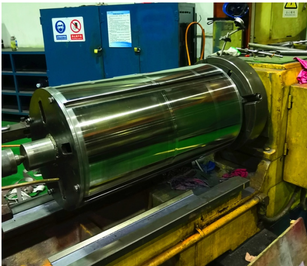
Figure 7: High Precision Machining - New S/T Bushes OD
