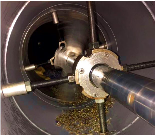
Figure 5: Line Boring In Progress
