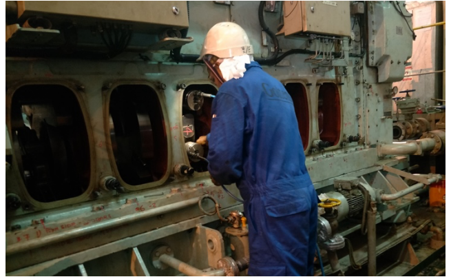
Figure 4: Hydraulic tensioning big end conrod bolts
