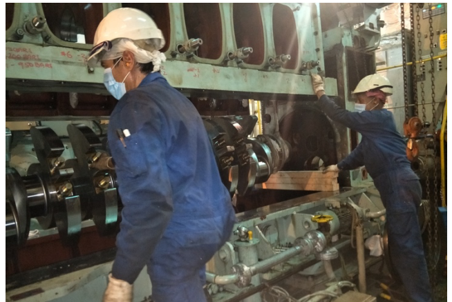
Figure 1: Block lifted, removing condemned crankshaft
