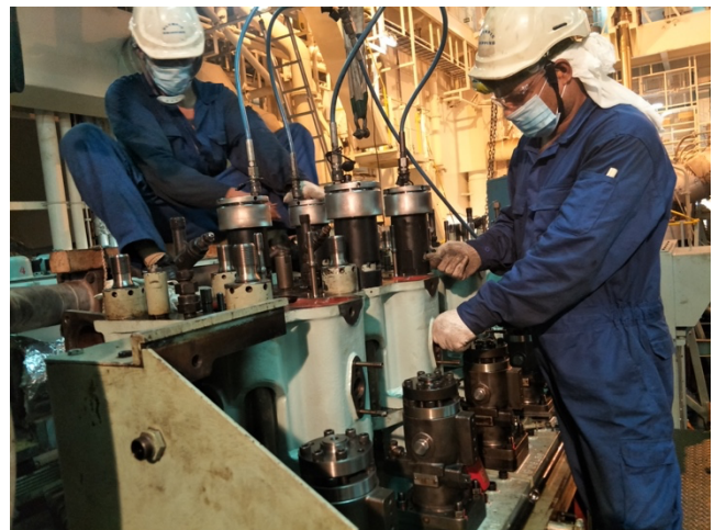
Figure 6: Hydraulic Tensioning of cylinder head studs
