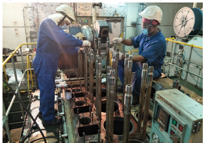
Figure 3: Torqueing of cylinder head studs
