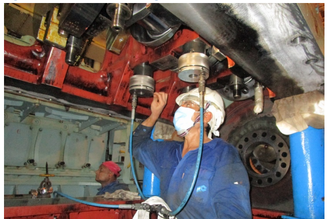
Figure 2: Hydraulic tensioning main journal bearing caps
