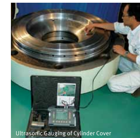
Ultrasonic Gauging of Cylinder Cover
