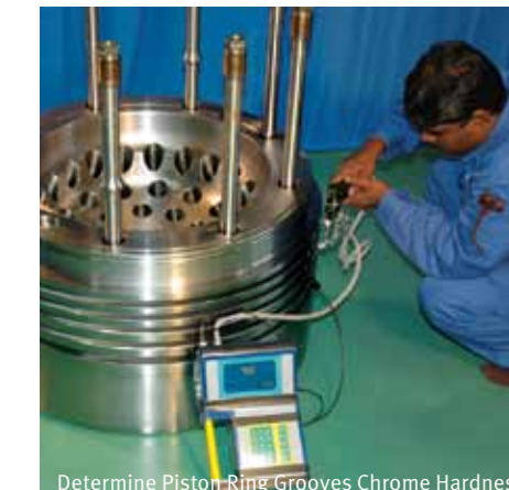
Determine Piston Ring Grooves Chrome Hardness
