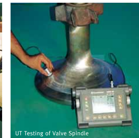
UT Testing of Valve Spindle
