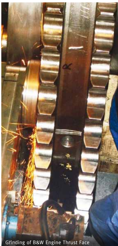
Multi Point Machining of Crankpin
