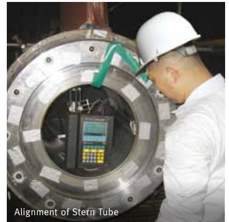
Laser Alignment Check of Propulsion Shaft Line
