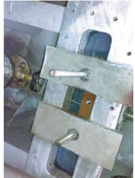
P' Bracket filled with Chockfast®
