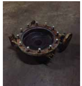
Refurbish damage rubber with Flexane
