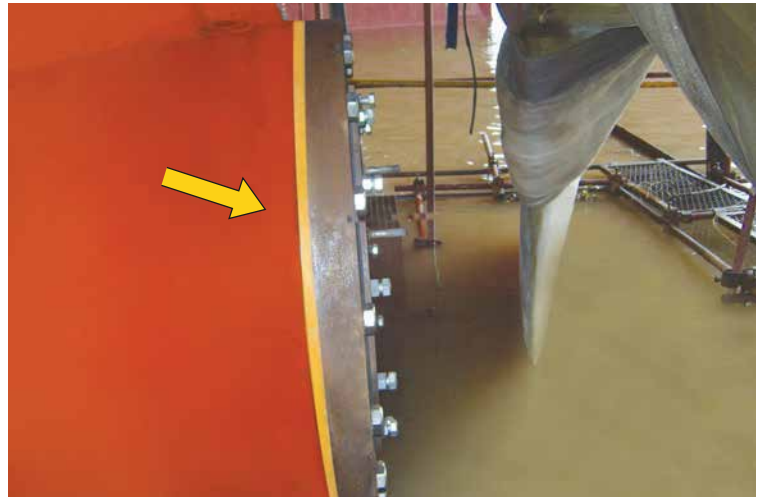
Phillybond orange provides water tight integrity on stern tube application
