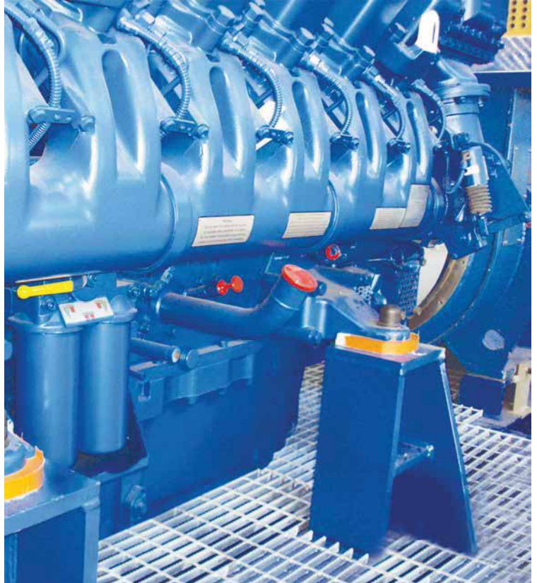
Chockfast® application on Auxiliary Engine
