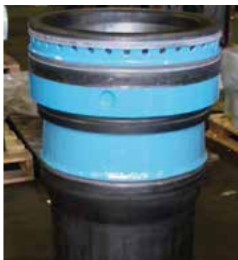
Brushable Ceramic promotes lifespan of cylinder liner
