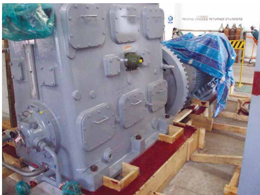
Industrial compressor motor with Chockfast®
