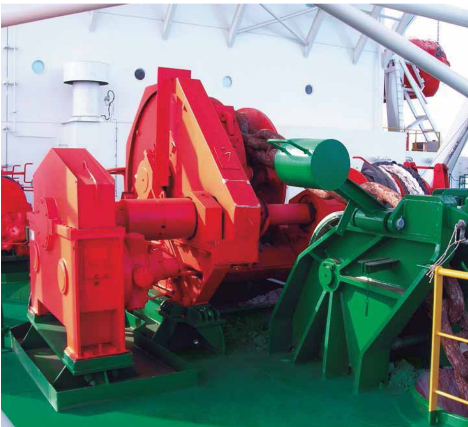
Anchor Windlass aligned and chocked with Chockfast®
