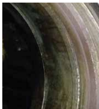
Devcon. in situ repair on engine block cylinder housing
