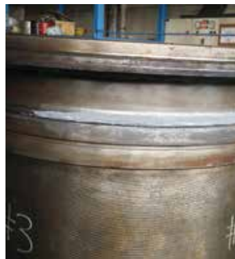
Completion of titanium application awaiting next process
