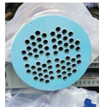
Preventive coat on new tubesheet
