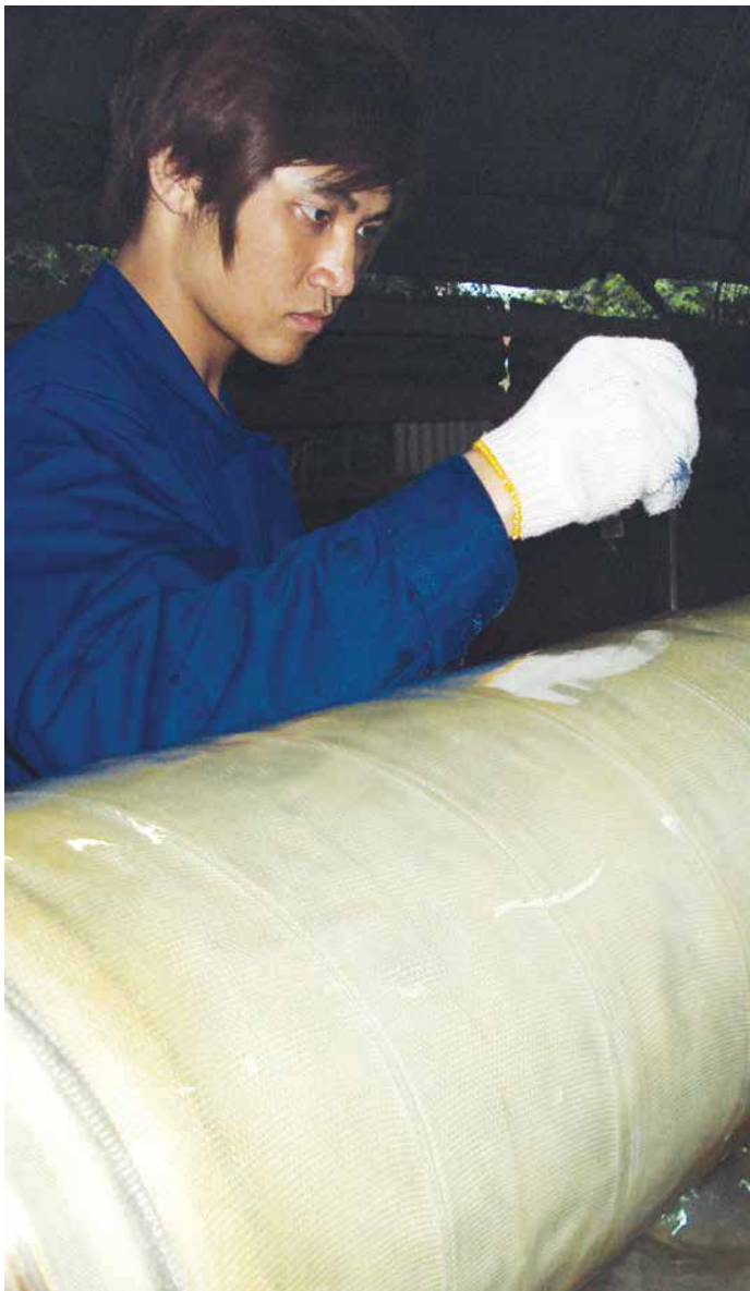
Checking on the Shaft surfaces to ensure even lamination
