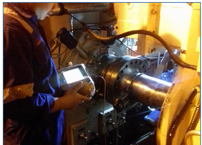
Laser alignment of generator to gearbox
