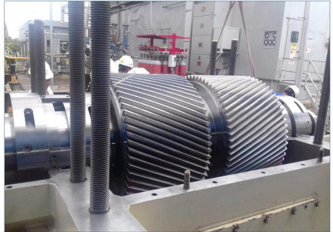
Gear teeth after repairs completed
