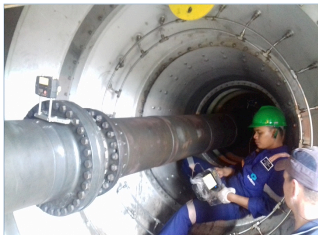
Laser alignment of generator to gearbox
