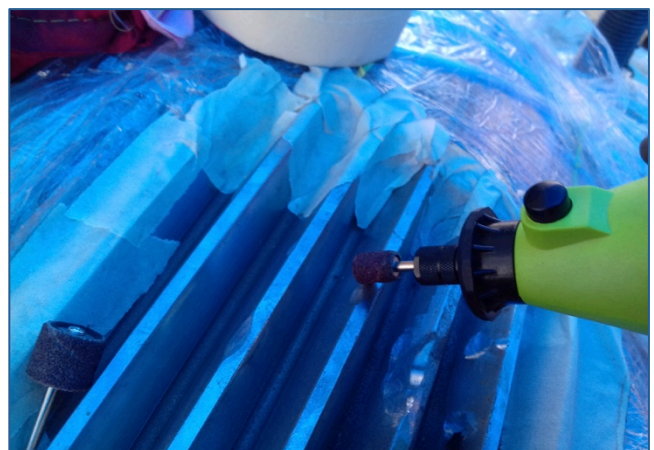
Pre-machining chipped gear teeth
