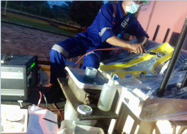
Selective electroplating damaged gear teeth
