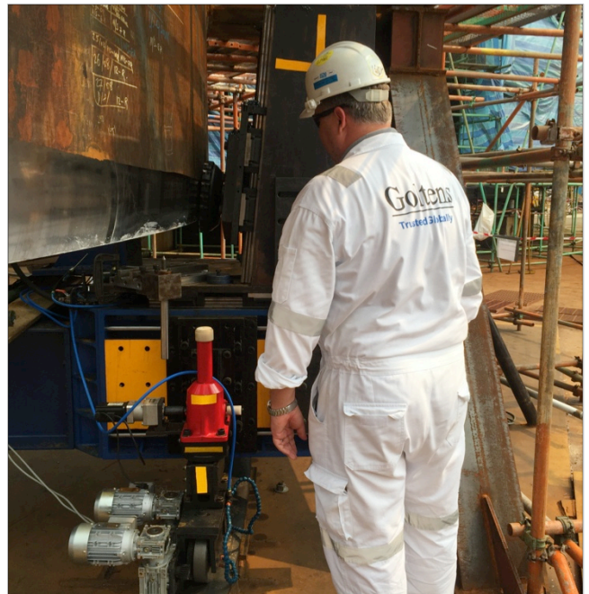
Machining lower outside diameter at 5.2° chamfer
