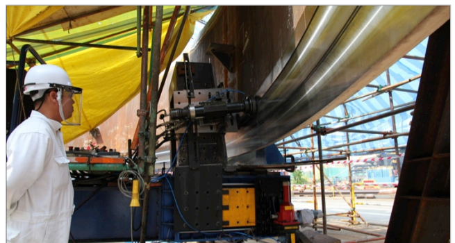
Machining lower inside diameter at 8.0° chamfer
