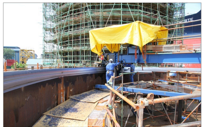
Machining top inside diameter at 5.2°
