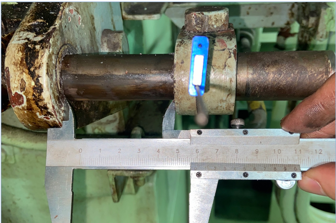
Re-set the governor data return to zero, re-measure the locked mechanical stopper real length
