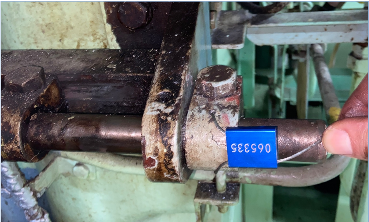
Drill hole and install the locked seal on mechanical stopper
