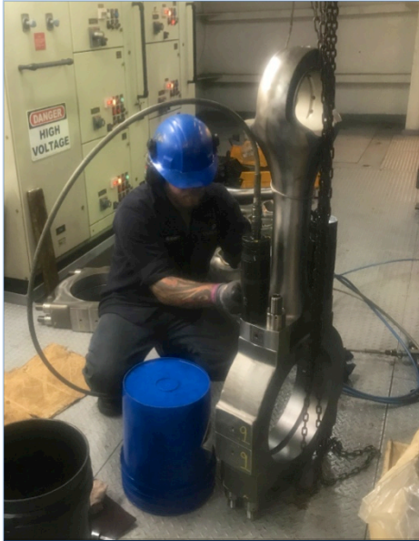
Calibration checks of piston rods under full torque
