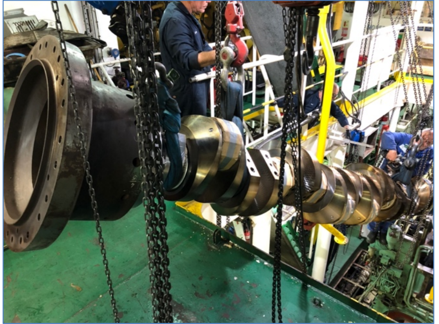
Figure 8: Goltens technicians rigging new crankshaft to lower engine room deck
