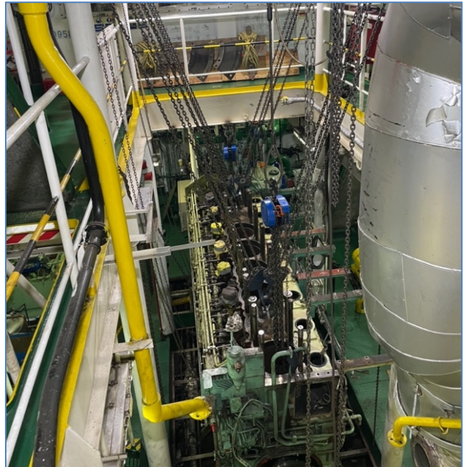
Figure 1: Engine stripped with rigging equipment attached to crankshaft for lowering
