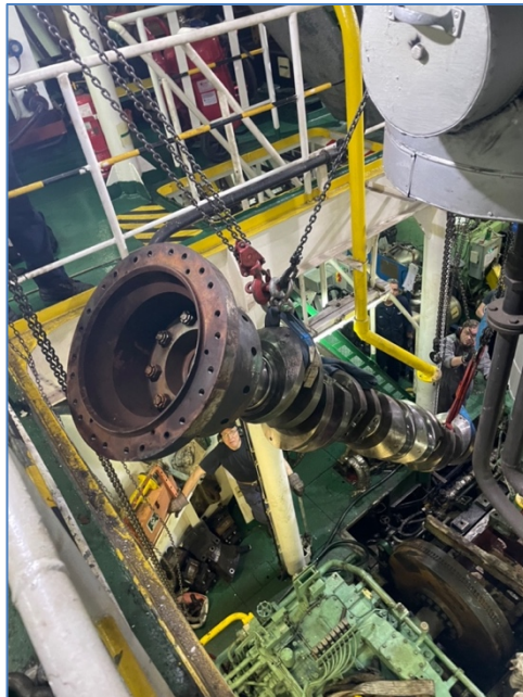
Figure 5: Rigging condemned shaft out of the engine room
