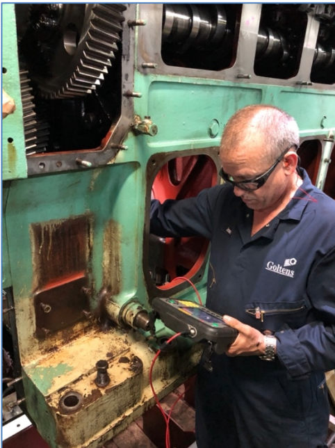
Figure 9: Laser check of block bore
