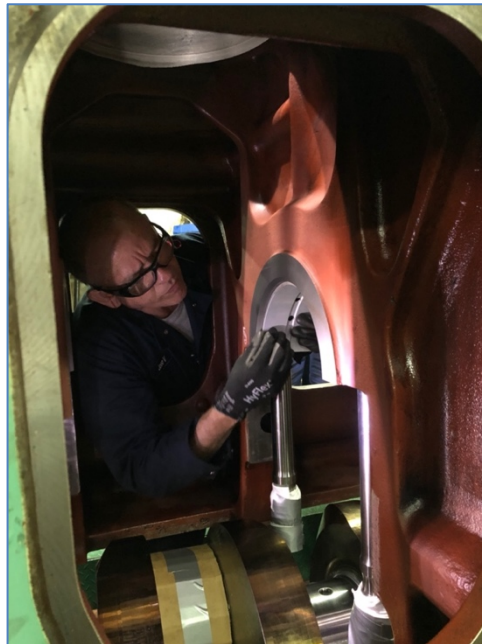
Figure 10: Installing new upper bearing shells before lifting crankshaft into position
