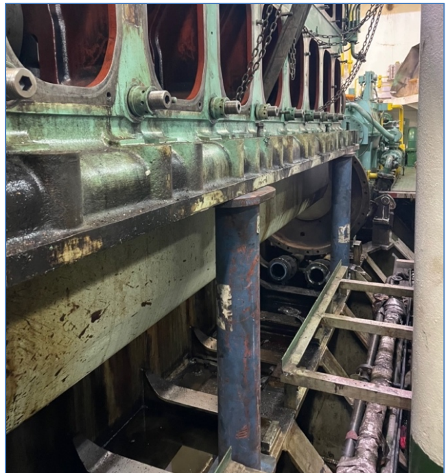
Figure 2: Engine block lifted and braced for crankshaft removal
