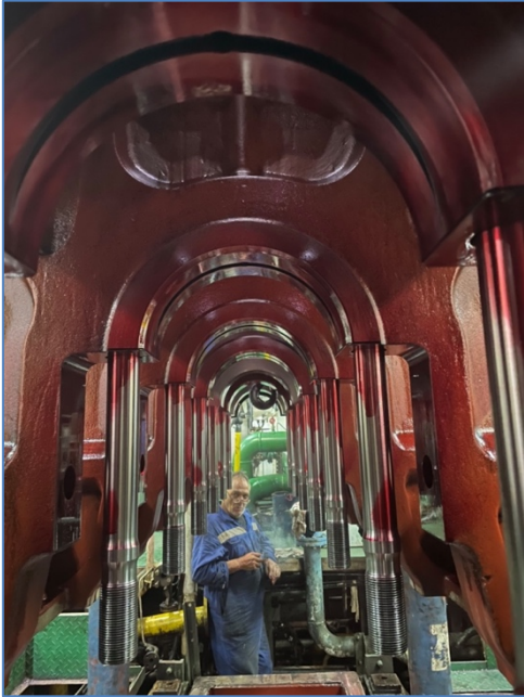
Figure 7: Non-Destructive crack testing on block prior to new crankshaft installation
