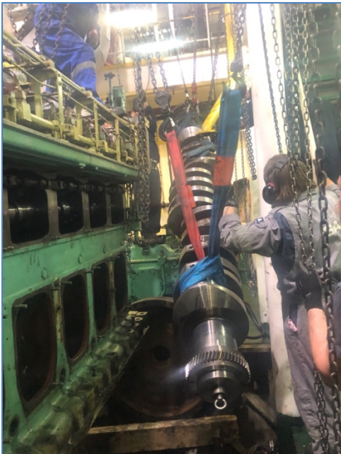
Figure 4: Crankshaft rigged from underneath block
