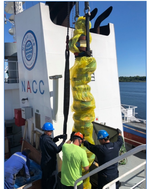
Figure 6: Lowering replacement crankshaft into the engine room with shore crane
