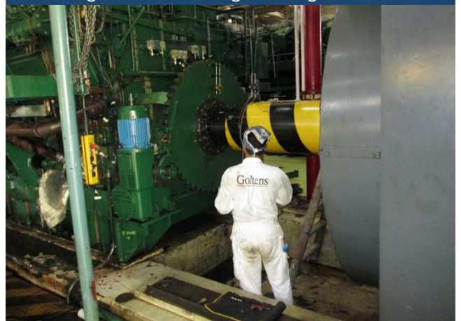
Laser alignment of the engine and generator
