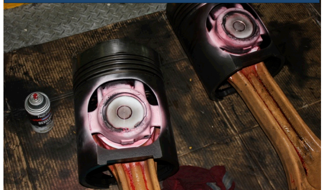
Calibration & crack checks on piston skirt
