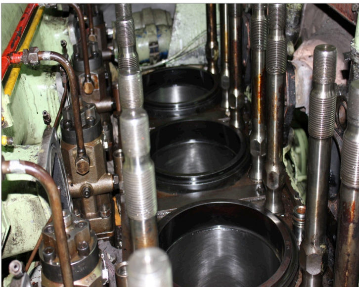
Liners- measured, honed, cleaned & installed
