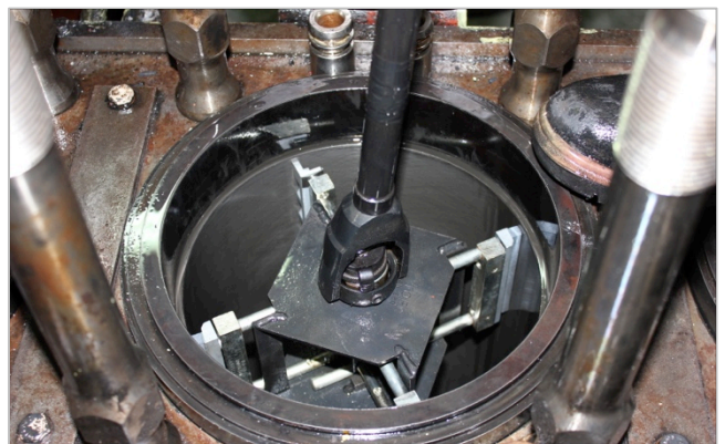
Honing of cylinder liners onboard
