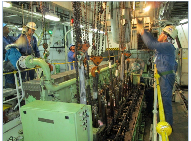
Lifting arrangements for block and crankshaft
