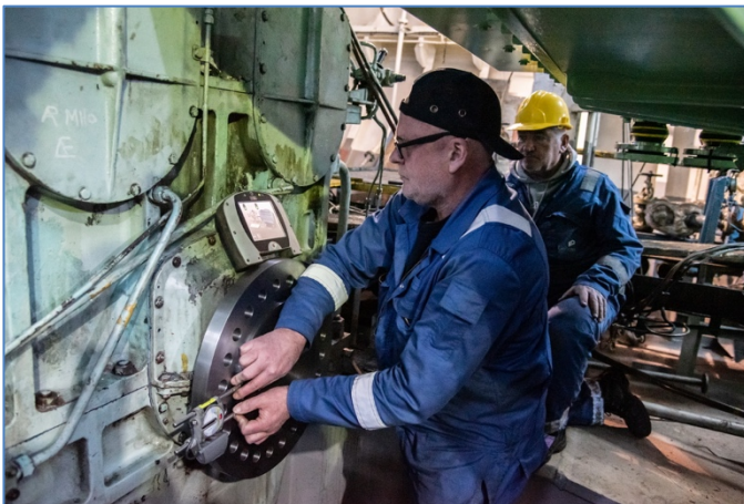
Figure 6: Laser alignment checks on engine and gear box
