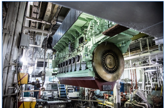
Figure 3: Lowering the engine into position above foundation
