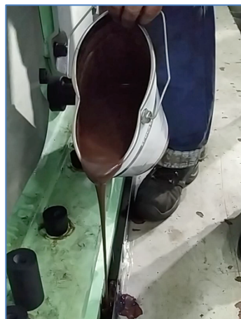
Figure 9: Chocking the engine
