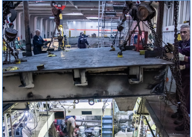
Figure 1: Removal of the deck to allow for engine rigging
