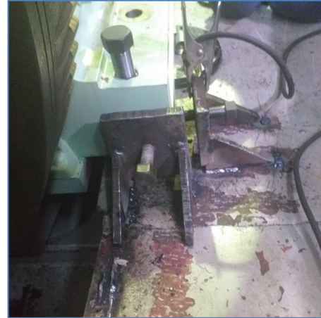
Figure 5: Jacking bolts installed
