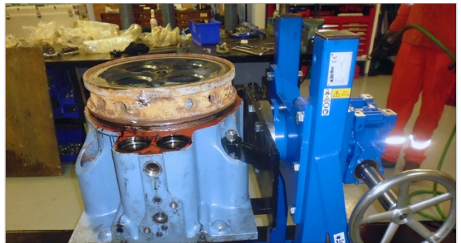
Inspection of cylinder head onboard vessel
