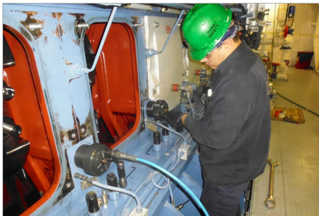
Torque main bearing side bolts
