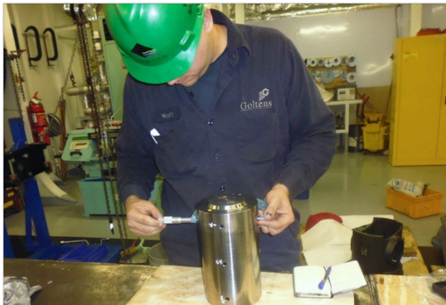
Measurement and inspection of piston pin
