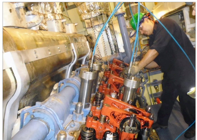
Checking hydraulic torque of cylinder heads
