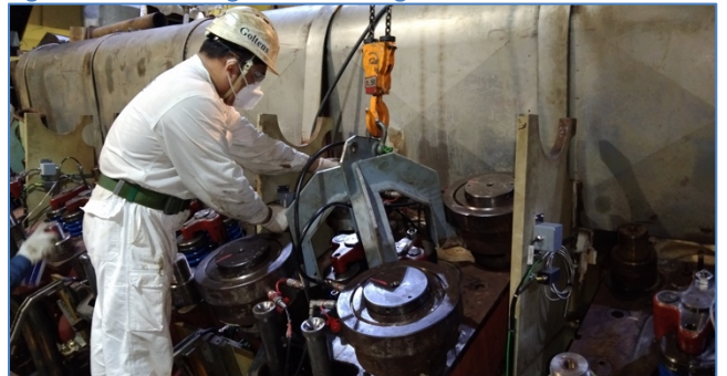
Figure 3: Slacking of Cylinder head nuts
