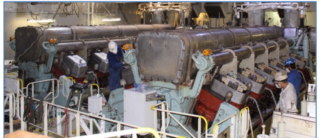
Figure 1: Goltens technicians disassembling one of the 12V50DFs
