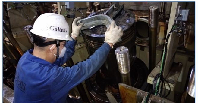
Figure 2: Goltens Engineer removing Piston
