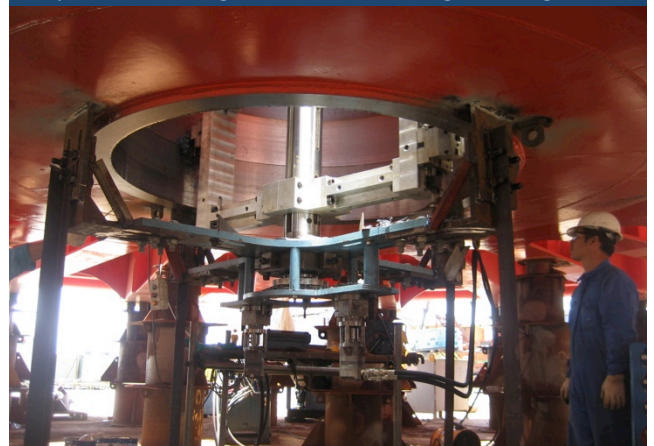
Taper line boring of bottom bearing housing
