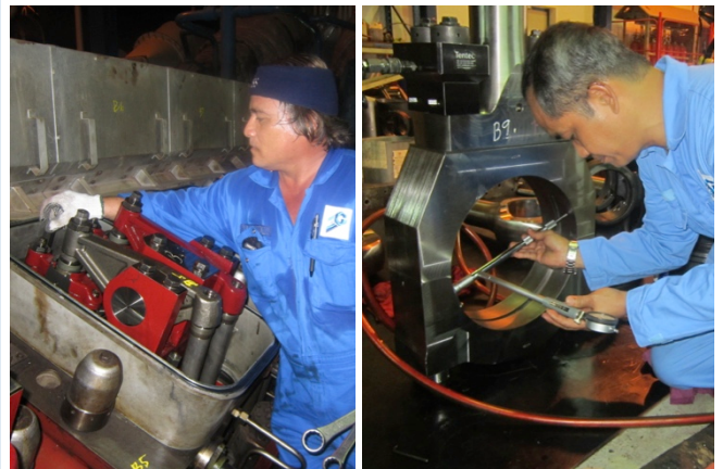
Installation of cylinder head and calibration checks on big end bearing housing
