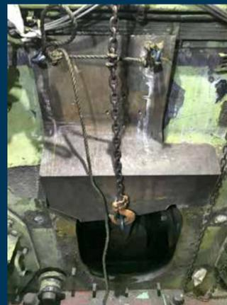
Cast and milled insert rigged into position
