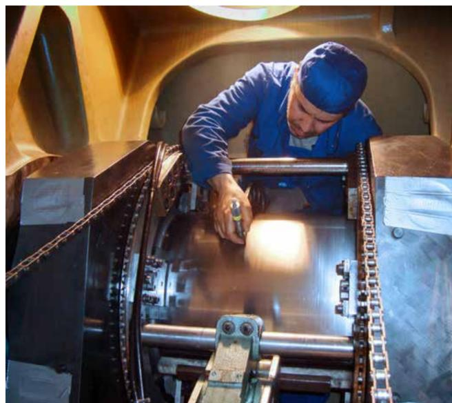
Checking journal diameter during finish machining
