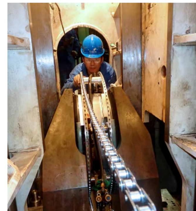
Finishing the machining of journal to -6.00mm
