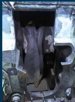
Crankcase damage cropped to insert dimensions
