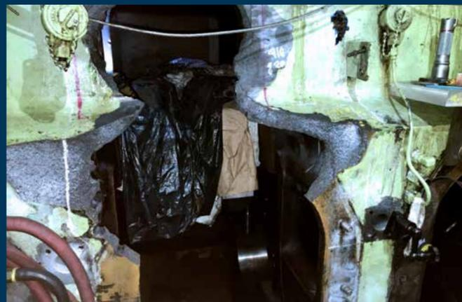
Crankcase exterior damage
