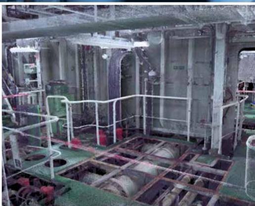
**2** The scan produces a point cloud of over ten million data points. For an average installation, 15 to 35 scans are made. These point clouds are stitched together and used by a 3D CAD program to create a fully three dimensional and highly accurate image of the area and all details inside it.
