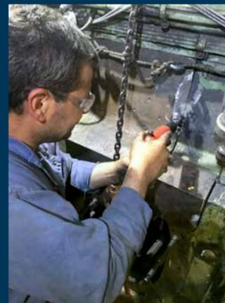
Drilling holes for stitch inserts along seam
