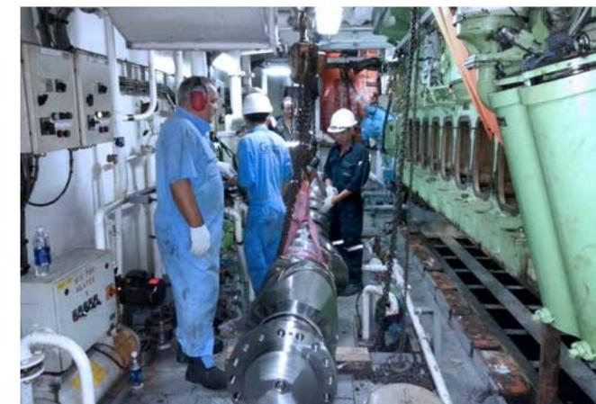
Block lifted with new crankshaft on deck ready for installation
