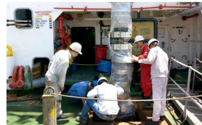
Replacement crankshaft being rigged onto the vessel for installation
