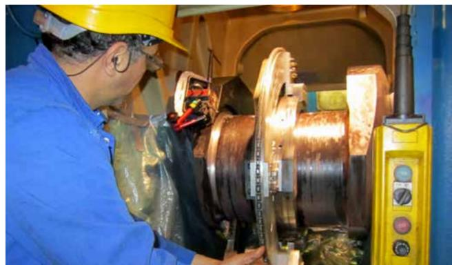
Machining the radius post annealing
