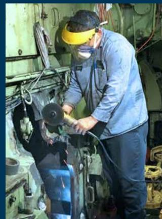
Cropping damaged section from crankcase
