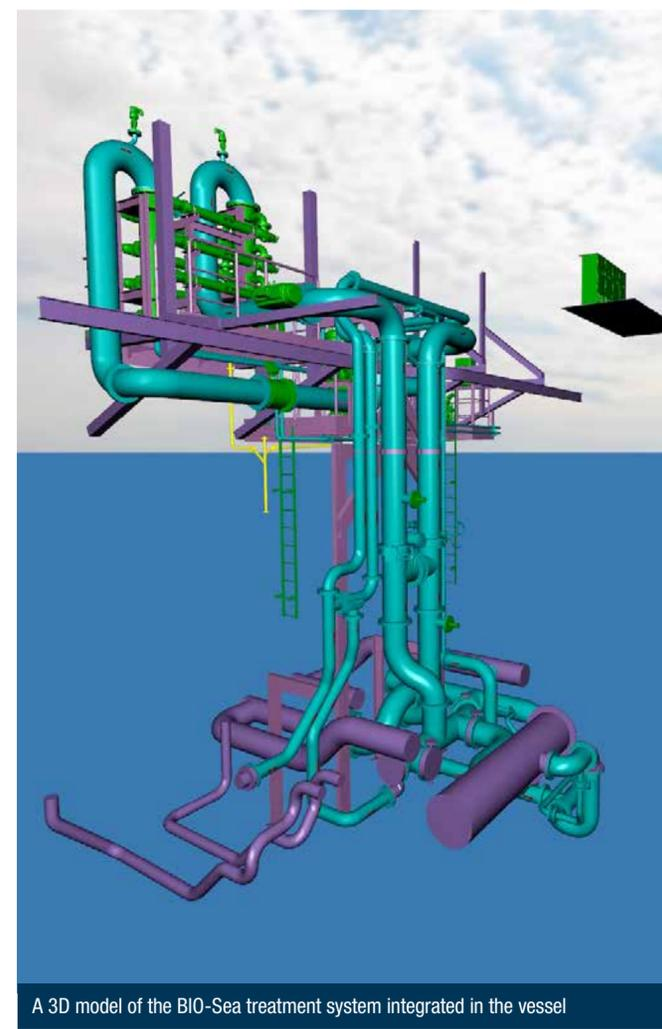
A 3D model of the BIO-Sea treatment system integrated in the vessel
