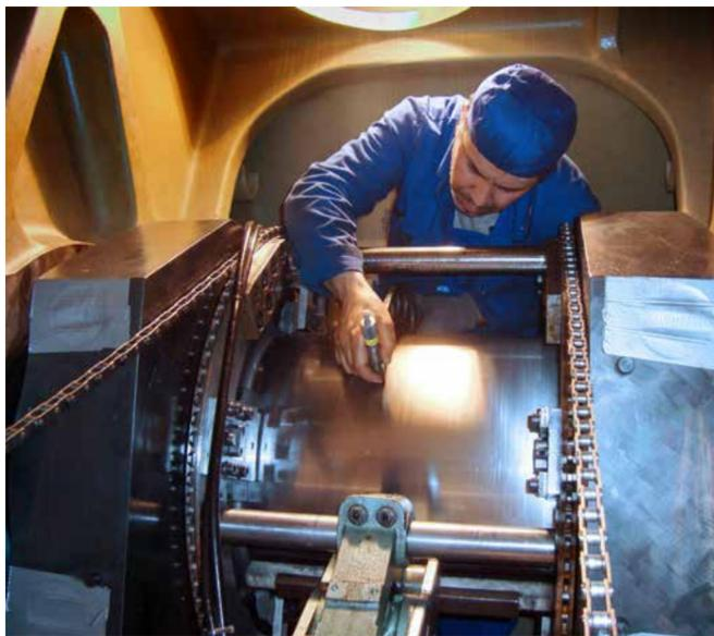
Checking journal diameter during finish machining
