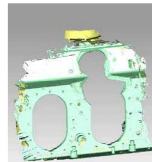
3D laser scan of the damaged portion
