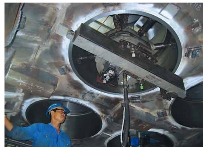
Flange facing in process on one of the 925mm lower gear box bores
