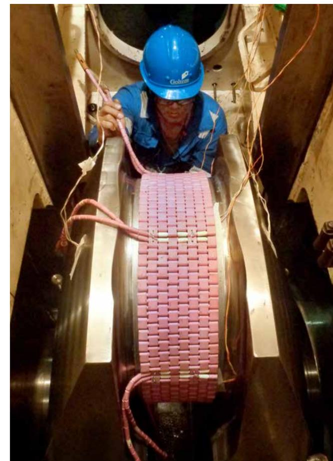
Installation of the annealing tiles on the damaged journal
