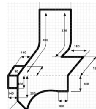
Design for cast insert and crankcase cropping
