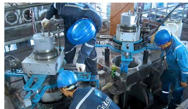
Multiple sets of boring equipment were used to speed the machining of the 36 925mm and 440mm top and bottom gear casing bores
