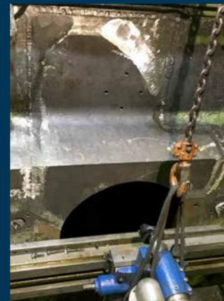
Stitching complete ahead of lock insertion and finish machining
