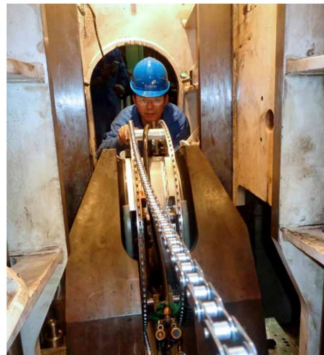
Finishing the machining of journal to -6.00mm
