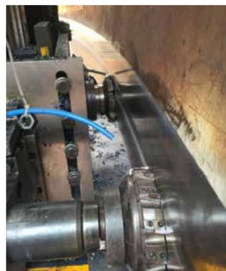
Two milling heads working at same time to maximize material removal
