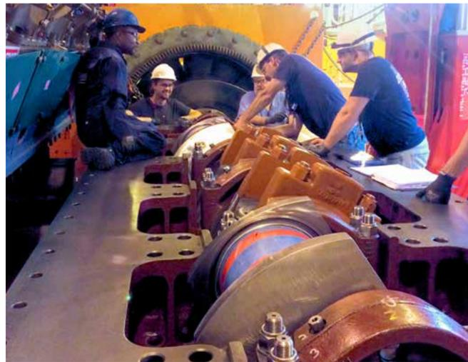
Replacement of bearing caps to check line bore
