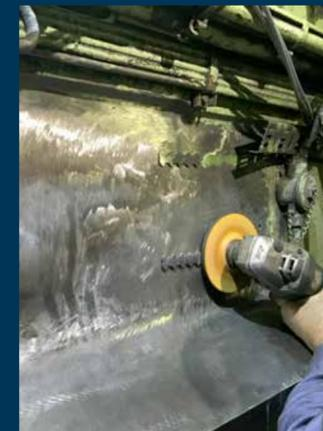
Final machining of crankcase surface after locks have been inserted
