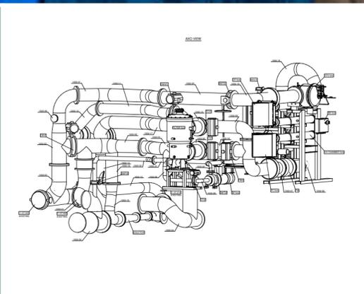
**5** The accuracy of the process allows for the prefabrication of a complete kit, ready for installation. Piping (including its pre-galvanizing), connections and foundations can also be precisely prefabricated, which eliminates the time-consuming, on-site pipe fitting process. This process is particularly attractive for sister vessel retrofits. Because the design can be re-used on sister vessels, overall costs will decrease for each vessel beyond the first.
