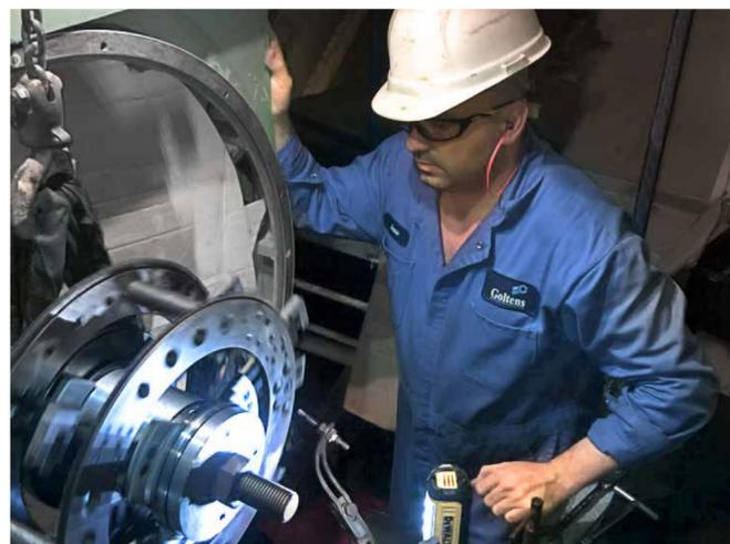
Goltens' new small range cutting tools in action on a 140mm diameter alternator shaft with 130mm between the rings. The shaft was machined to 130.00mm and a sleeve insert was installed to oversize at 141.00. Shaft was then finish machined to 140.00mm. The job was completed in only five days.
