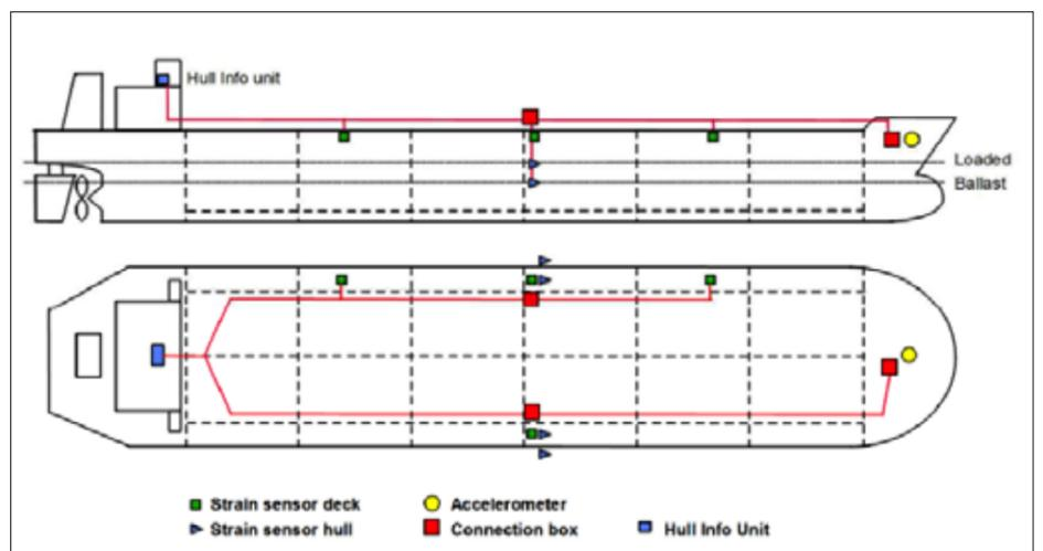
Representative component placement for hull condition monitoring components
