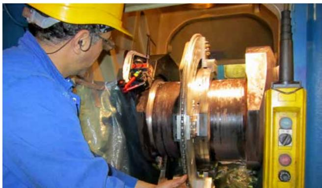
Machining the radius post annealing
