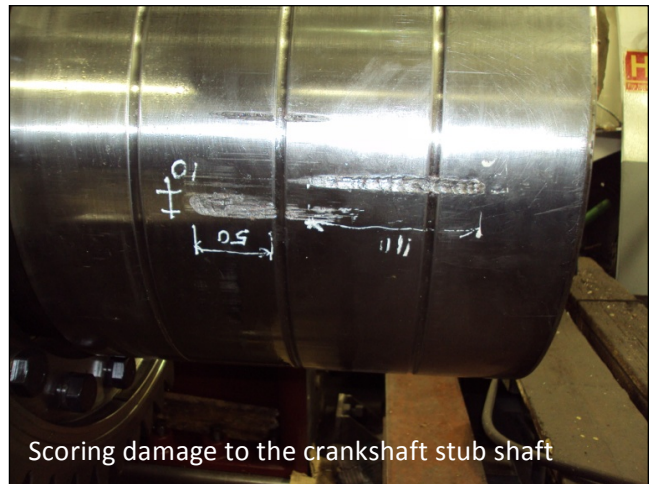
Machining damaged area from journal surface
