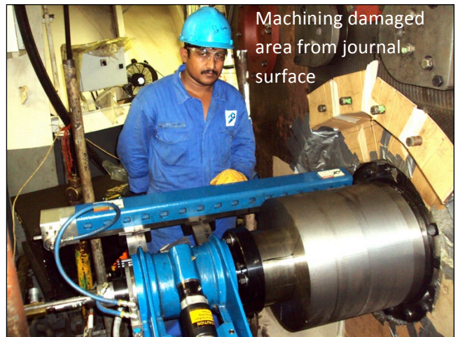
Machined shaft surface (-4mm) pre-machining of oil grooves in the shaft
