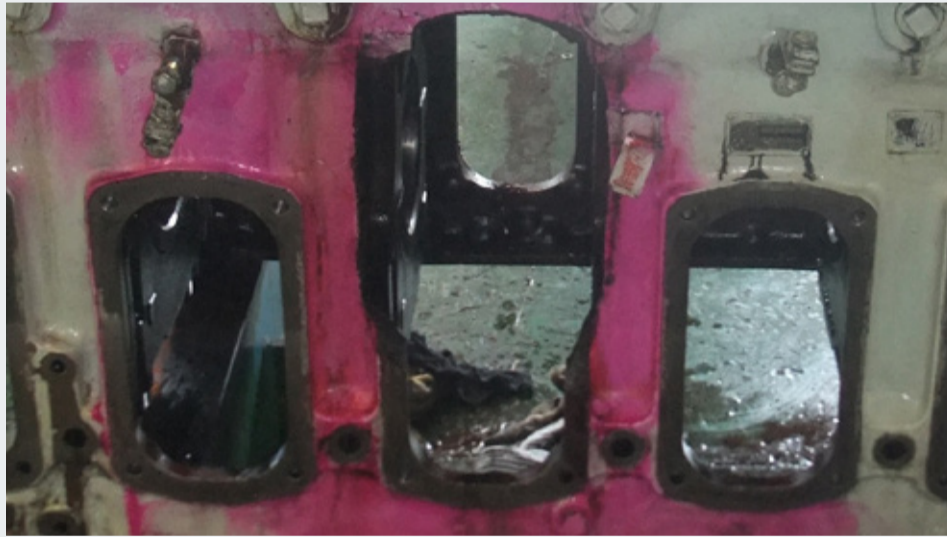
Badly damaged Yanmar 6N18-UN crankcase door resulting from a connecting rod failure.
