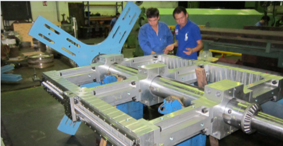
Goltens' G2000 boring machine during construction in Goltens Singapore workshop.
