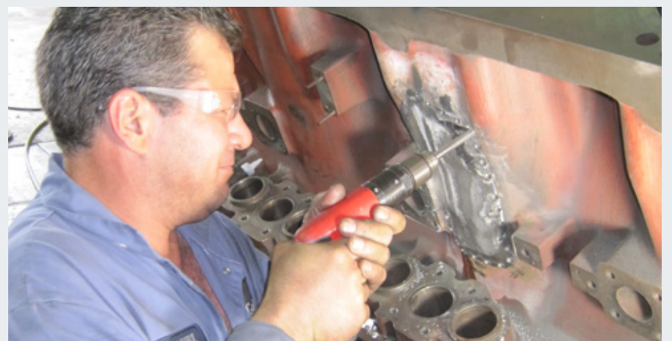
Goltens' machinist stitching replacement piece into place prior to installation of locks to complete the repair.
