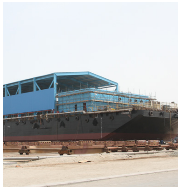
Docking scope is complete along with total refurbishment of the structure housing the desalination equipment.
