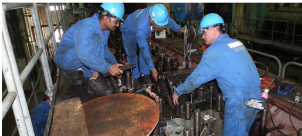
Goltens' Diesel Technicians fastening the lifting yoke to remove a cylinder head from one of the MAN B&W engines.
