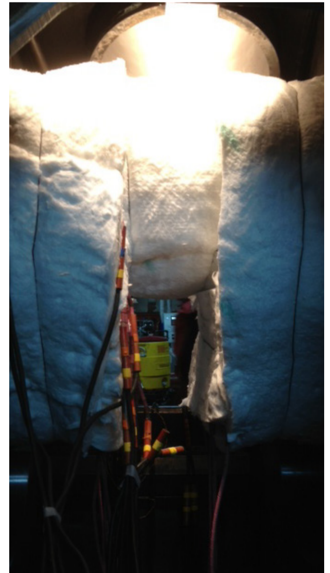
Annealing equipment installed and insulated on the damaged pin after machining to remove all surface cracks.
