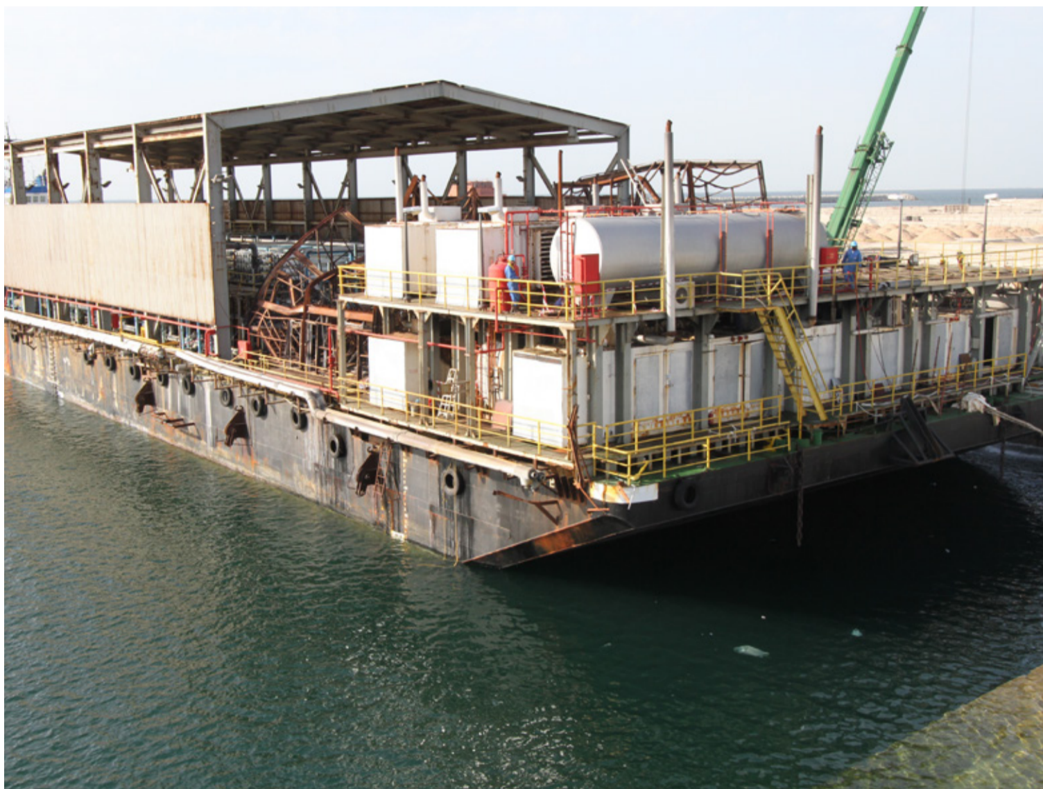
Bowarege 2 arrives in DMC end December 2013 with its Accommodation Block completely destroyed as well as serious damage to several containerized Gensets
