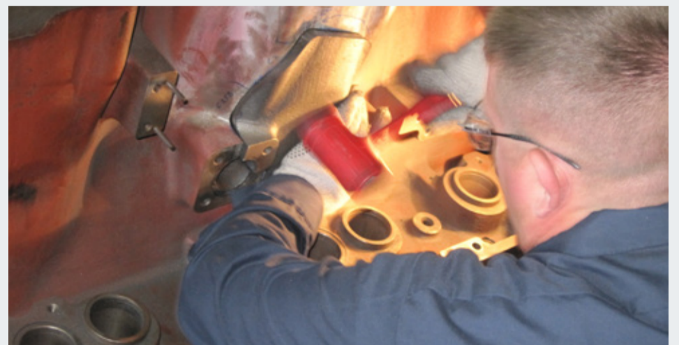
Machinist fitting replacement piece into place prior to metal stitching.
