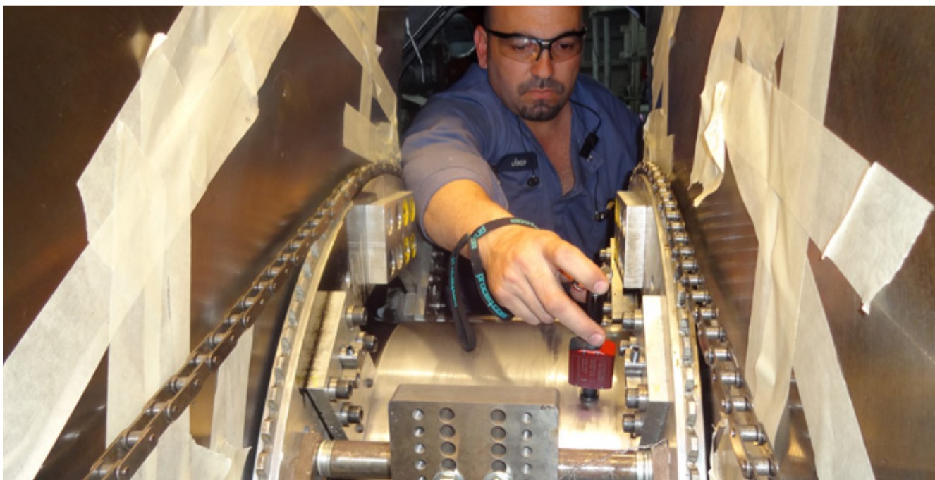
Checking journal hardness before annealing after machining 0.40mm from the damaged surface on the Rappahannock's PIELSTICK 10PC4.2V main engine.
