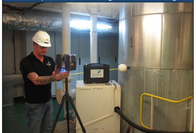
Goltens specialist conducting 3D laser scanning
