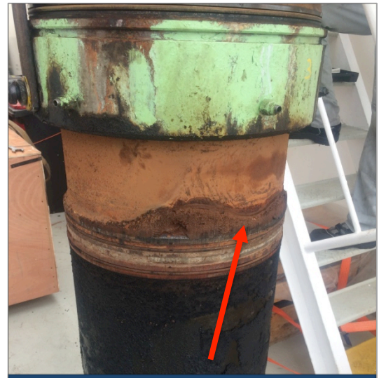
Significant sediment build up on lower liner
